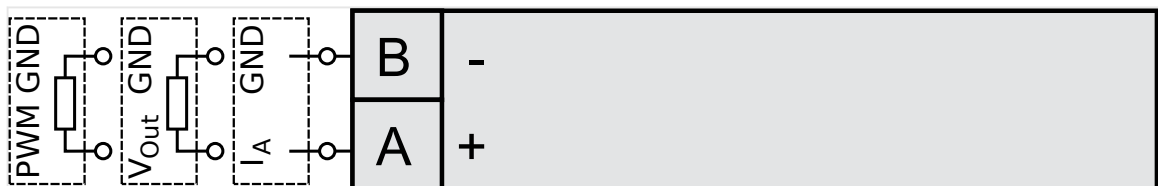
Fig. 58: Analog controller output - two wires
