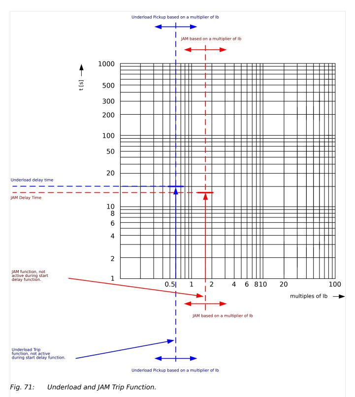
These would be represented by two such vertical lines, both below the normal load current. Be sure to set the alarm level *above* the trip level. Each element has its own delay timer. Use the start delay to block tripping until the load stabilizes after a start. Use run delays to avoid false alarms or trips for load transients.
