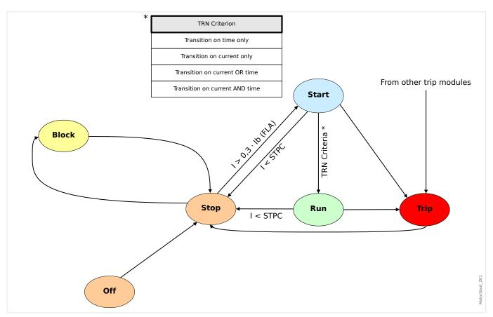
The basic motor operation states can be classified as four states that include:
