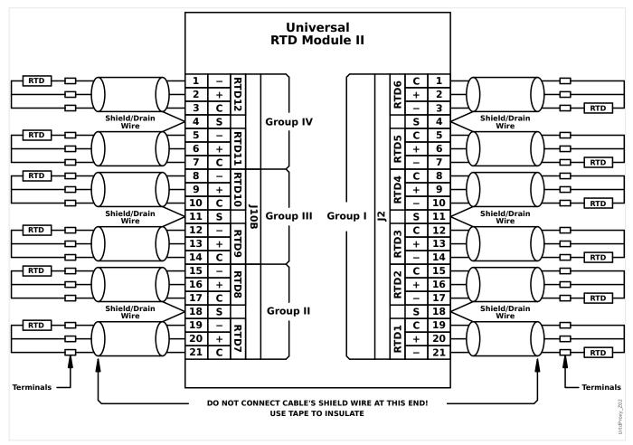
See the figure above for wiring of RTDs to the URTD inputs. Use three-conductor shielded cable. Note the connection rules in the figure. When making connections to a two-lead RTD, connect two of the cable conductors to one of the RTD leads as shown. Make this connection as close to the protected object as possible. Connect the third cable conductor to the remaining RTD lead.
