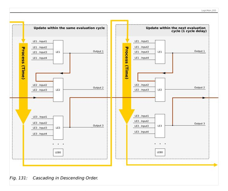
In the example shown in  $\sqsubseteq$  Fig. 131 above, "Logic Equation **2**" uses the output states of two other equations, "Logic Equation **1**" and "Logic Equation **3**". The result of "Logic Equation **1**" is used in ascending order and has therefore been evaluated within the same process cycle. The result of "Logic Equation **3**" is used in descending order and has therefore been evaluated in the previous process cycle.
