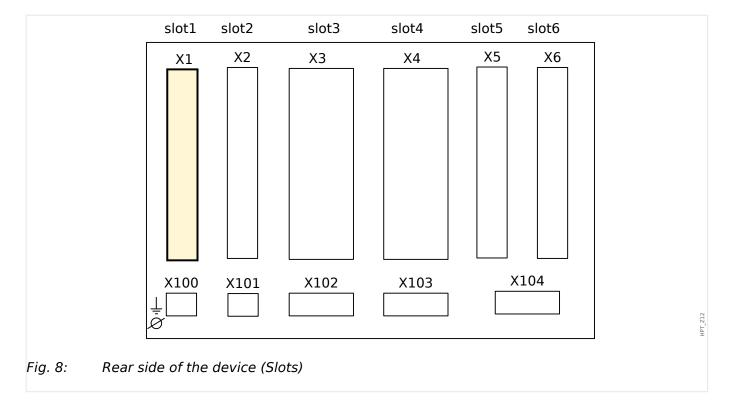
Power Supply Card with Digital Inputs
