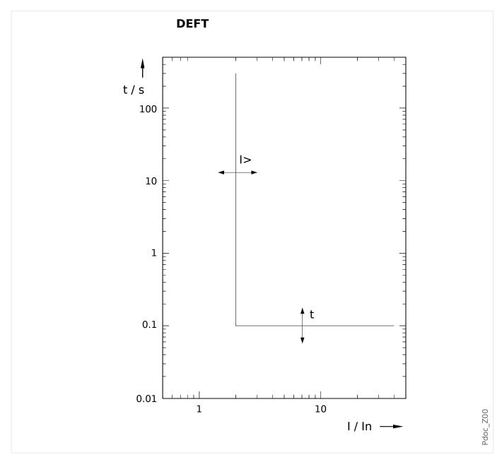
Trip delay for I > I>, settable via [Protection Para / Set 1...4 / I-Prot / I[x]] \*t«. The reset delay for I < I> always equals 0 ("instantaneous").
