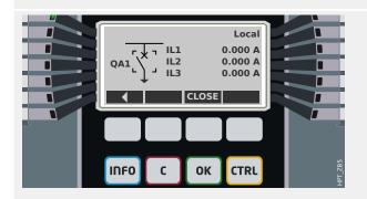
The Softkey "▶" (Enter) takes you to an enhanced single line (after you have entered the password for access level "Control-Lv1"). The switchgear device is highlighted by small markers (and in case of several implemented switchgear devices, the Softkey "Select" is visible, which allows you to select another one).
