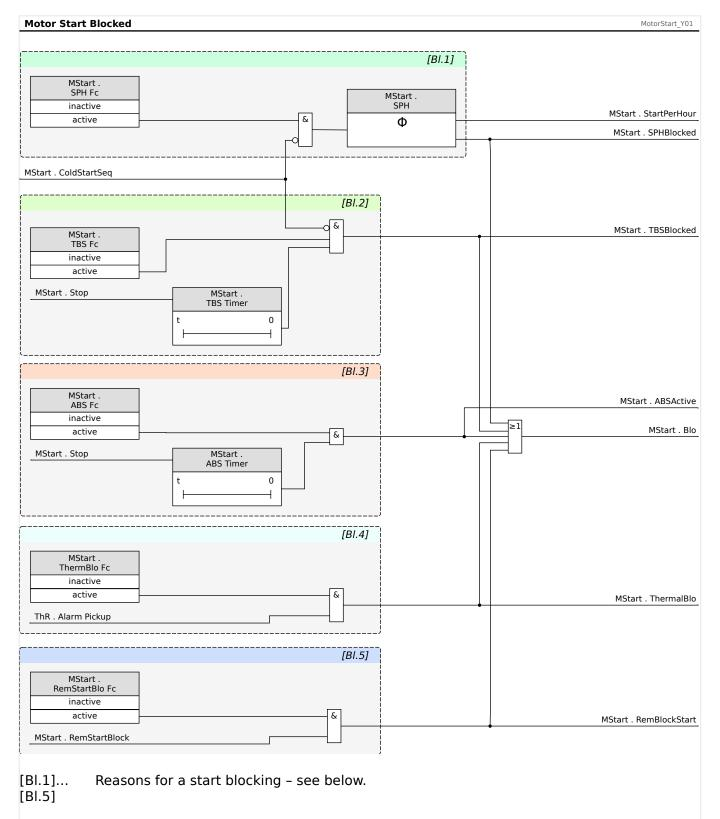
A Motor Start can be blocked by certain events, if any of the following conditions are noted – motor starts limit, starting frequency, thermal and mechanical constraints. The user may choose to use the states to block the motor from starting or use it as an alarm or indication. The reasons for a Motor Start Blocking can be as follows:
