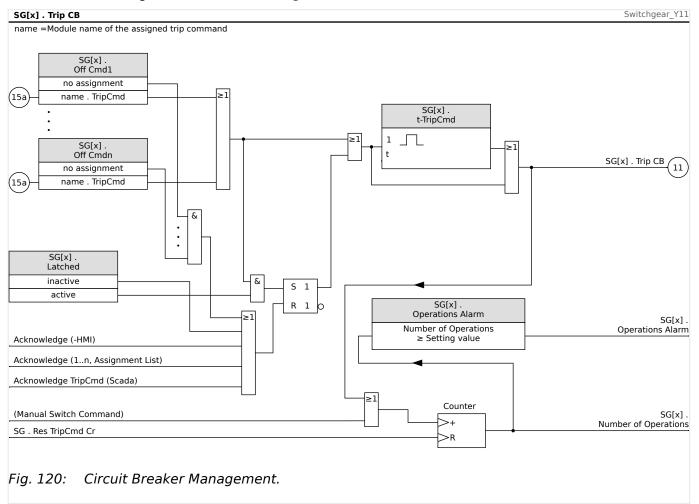
Note that in the diagram above, "SG[x]" represents "switchgear number x"; however, the exact designation is defined in the single-line file, see also  $\square$  "Single-Line Diagram".
