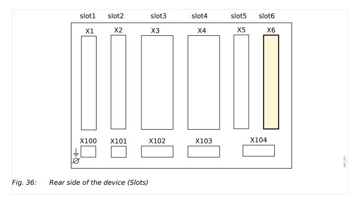
The type of card in this slot is dependent on the ordered device type. The different variants have a different scope of functions.
