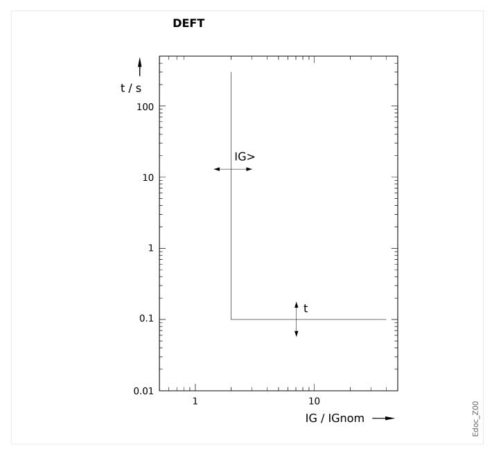
Trip delay for IG > IG>, settable via [Protection Para / Set 1...4 / I-Prot / IG[x]] »t«. The reset delay for IG < IG> always equals 0 ("instantaneous").
