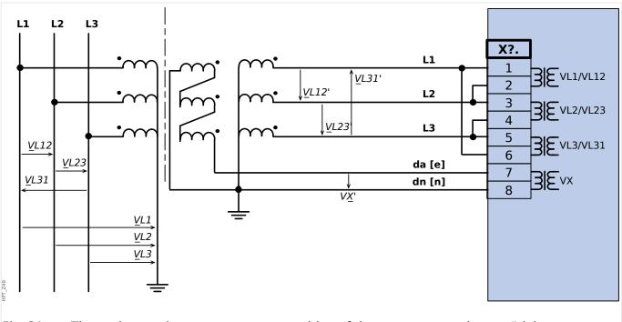
*Fig. 31:* Three-phase voltage measurement - wiring of the measurement inputs: "deltaconnection"Measurement of the residual voltage VG via auxilliary windings (e-n) "broken delta"
