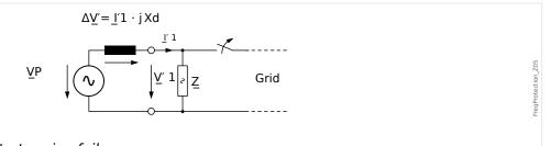
Fig. 105: Equivalent circuit at mains failure.
