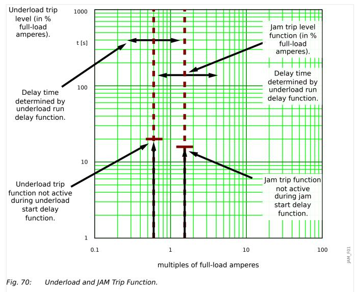
The MRMV4 issues an alarm when the pickup [Protection Para / Set 1...4 / JAM-Prot / Jam[x]] »Pickup« is exceeded. If the timer [Device planning] Jam[x]. »Mode« = "active" and [Protection Para / Set 1...4 / JAM-Prot / Jam[x]] »t« has elapsed, a trip signal will be issued.
