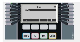
The Softkey "SG" takes you to a screen that lists all connected switchgear devices.
