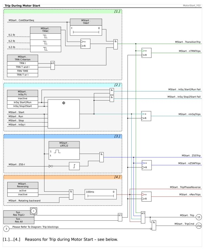
The motor is tripped during the start phase, in case that any of the following occurs:
