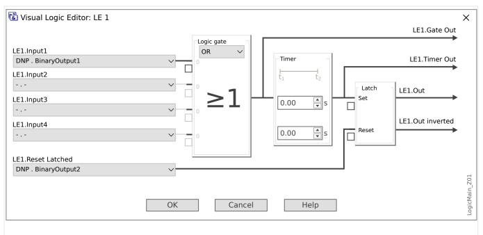
*Fig. 55:* Setting example from Smart view, to make a steady state signal from a DNP output signal.
