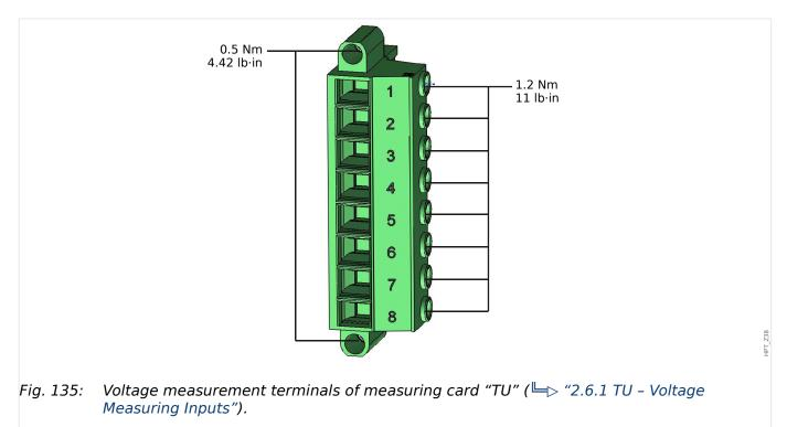
Voltage and Residual Voltage Measurement ("TU")
