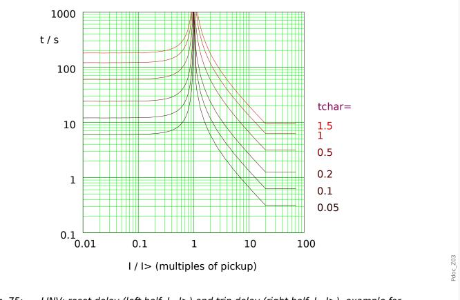
*Fig. 75:* LINV: reset delay (left half, I < I >) and trip delay (right half, I > I >), example for  $I_{max} = 20 \cdot I >$ .
