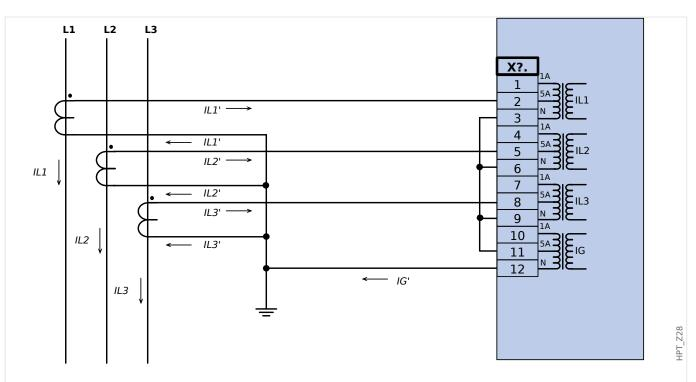
*Fig. 21:* Three phase current measurement; In secondary = 5 A. Earth-current measuring via Holmgreen-connection; IGnom secondary = 5 A.
