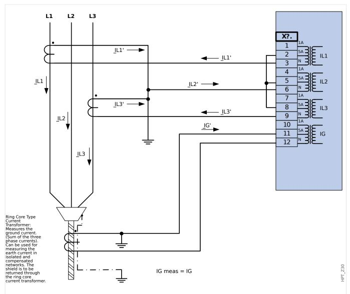
*Fig. 23:* Two phase current measurement (Open Delta); In secondary = 5 A. Earth-current measuring via cable-type current transformer ; IGnom secondary = 5 A.
