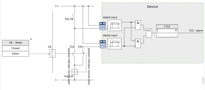
Fig. 112: Connection example: Trip circuit supervision with two CB auxiliary contacts »Aux ON« (52a) and »Aux OFF« (52b).
