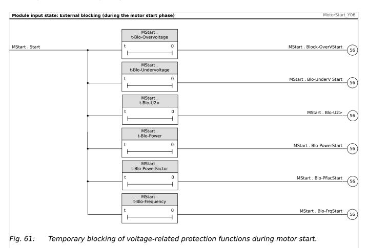
The setting parameters for all these start delays are available within the menu [Protection Para / Global Prot Para / MStart / Start Delay Timer].
