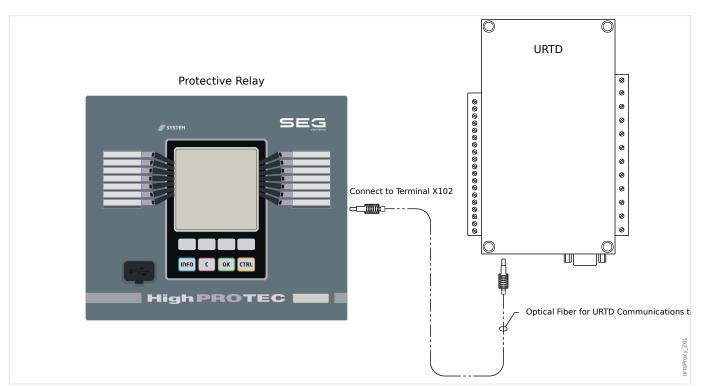
The figure above shows the fiber optic connections between the URTDII Module and the protective device. The protective device supports the optical fiber connection.
