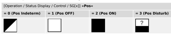
Assignment of Position Indications (Digital Inputs)
