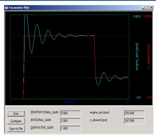
The application will read the previously saved configuration and request the controller to start sending the parameter values. The controller sends the data to the PC at a rate that varies with the number of parameters being monitored. The application uses the Windows timer functionality to update the screen at the specified rate. Note that if the PC is very busy, the timer accuracy will vary; therefore, the screen and generated data files should be considered as reference only.
