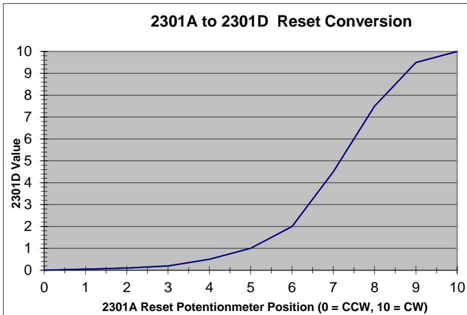
Figure B-2. Reset Potentiometer Conversion Chart
