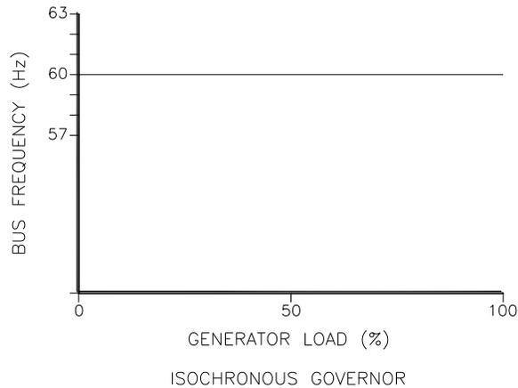
Figure 3-6. Isochronous Mode
