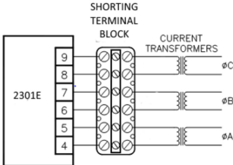
Figure 5-1. Temporary Wiring for Transformer Phase Correction
