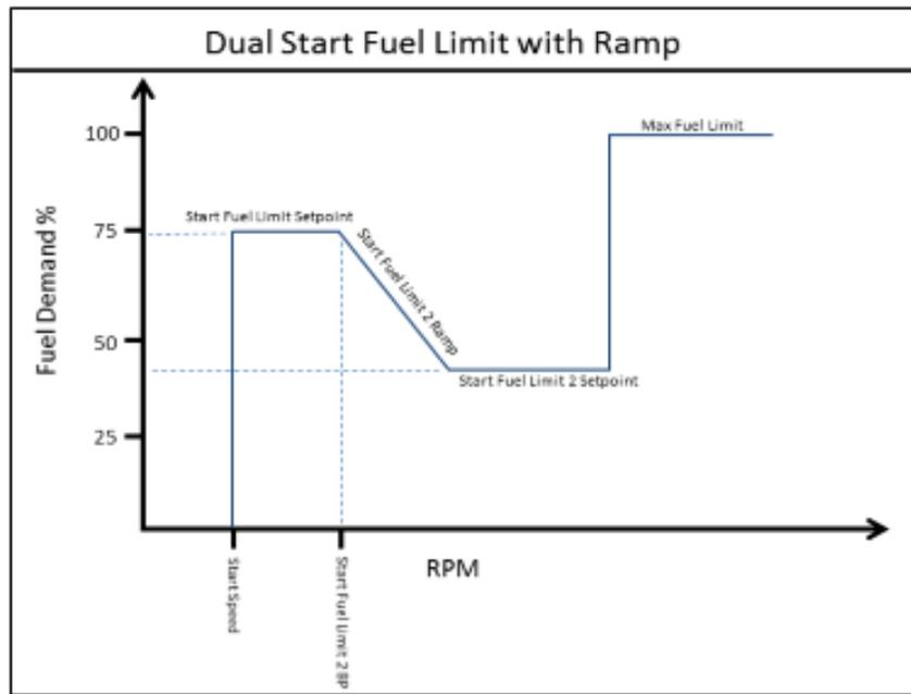
Figure 4-12. Dual Start Fuel Limit with Ramp
