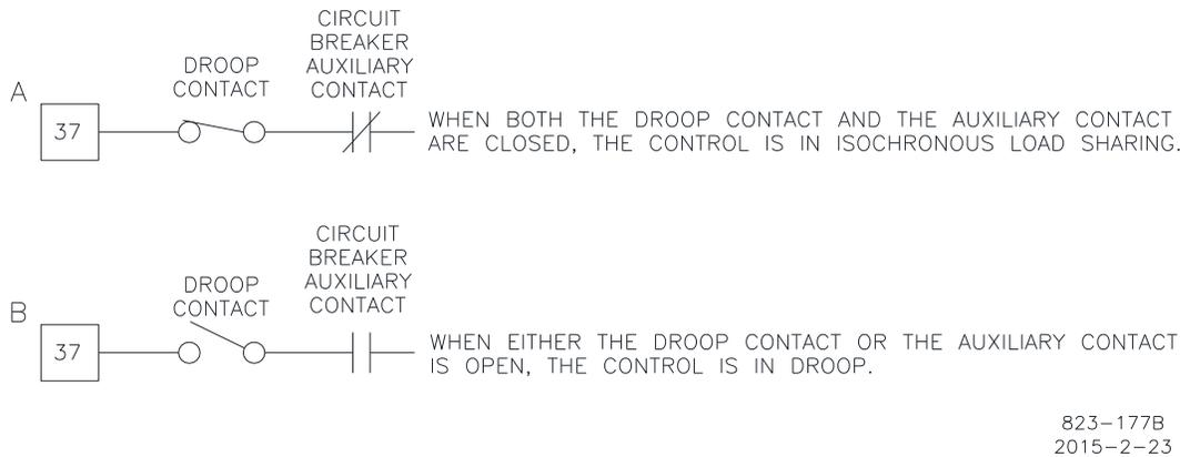
Figure 2-2. Droop Contact and Circuit Breaker Auxiliary Contact
