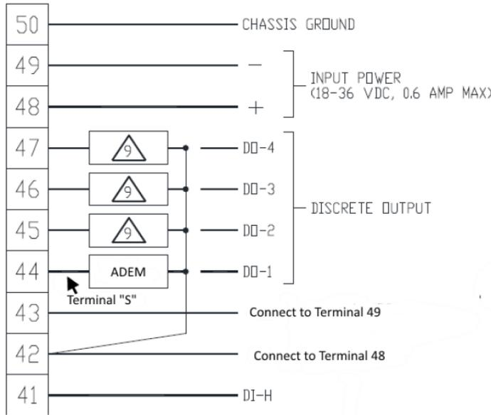
2.0 In the 2301E Configuration Mode, select the Actuator Output Type to 4. This activates Discrete Output #1 for a PWM output.
