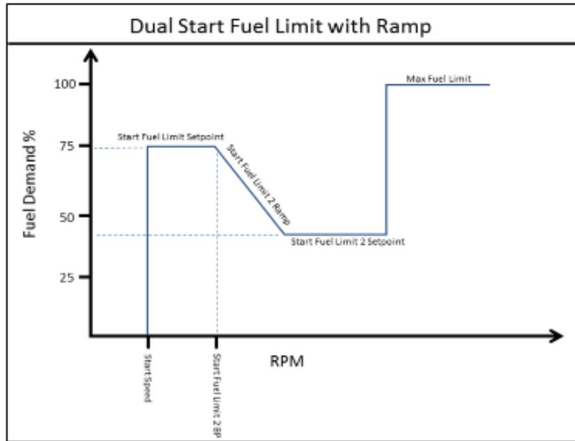
Figure 3-3. Dual Start Limit Function
