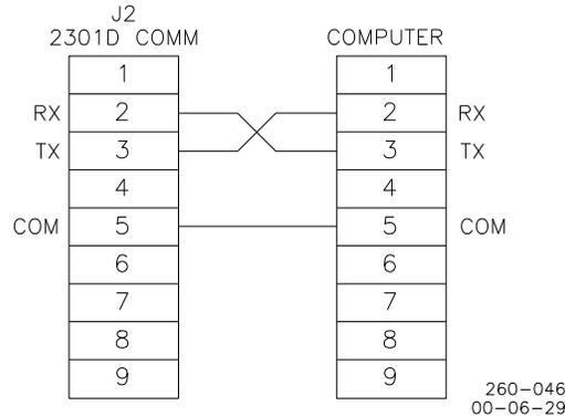
Figure 4-1. Null Modem Cable
