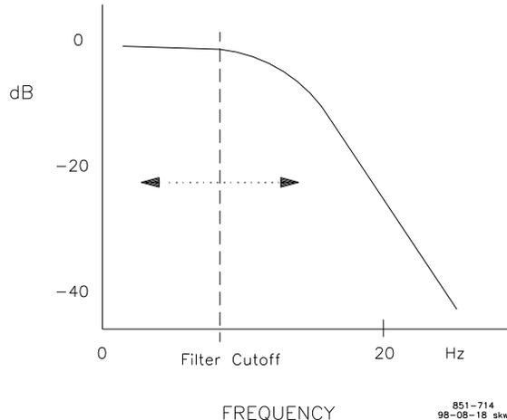
Figure 4-4. Speed Filter
