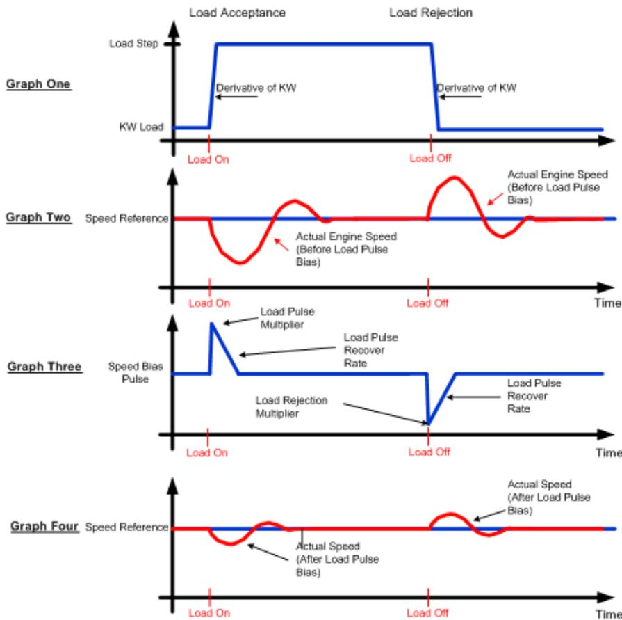
Figure 3-9. Load Pulse / Rejection
