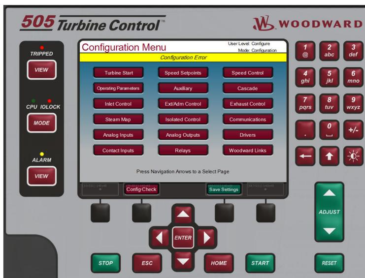
Figure 4-2. Configuration Menu – Configuration Mode (Edit)
