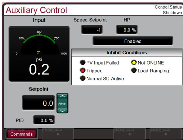
Figure 5-15. Auxiliary Control Screen
