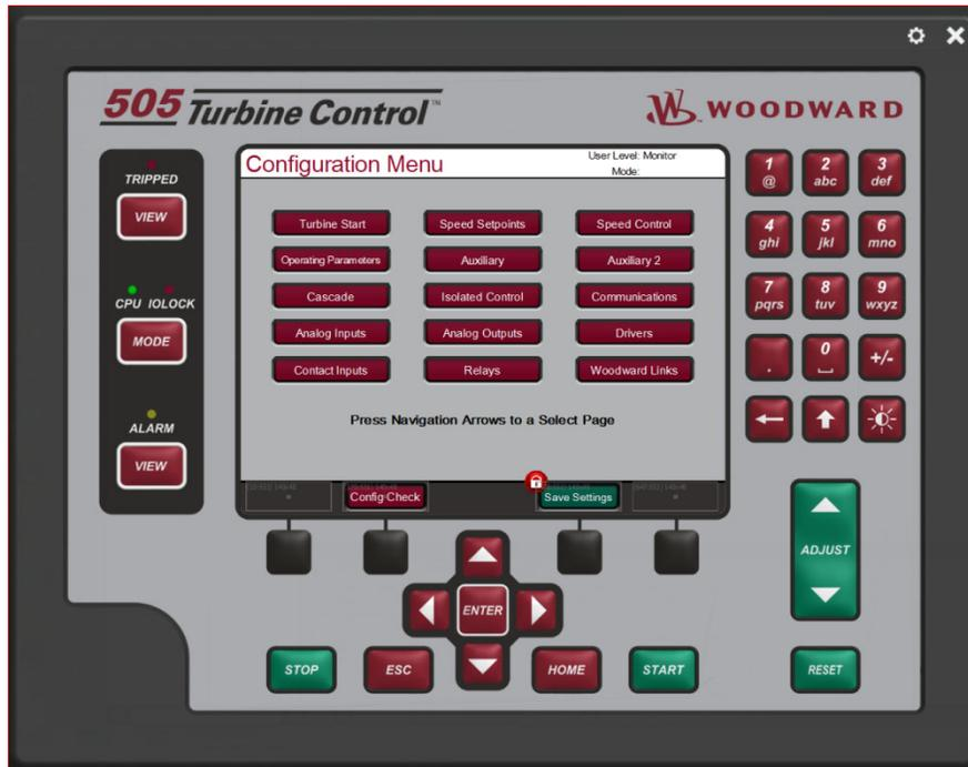
Figure 1-4. 505 Keypad and Display
