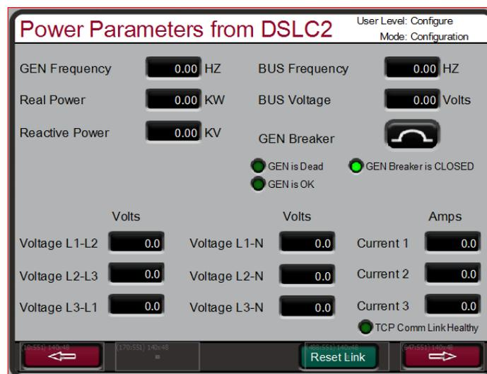
Figure 9-3. Service Screen - DSLC-2 Power Parameters
