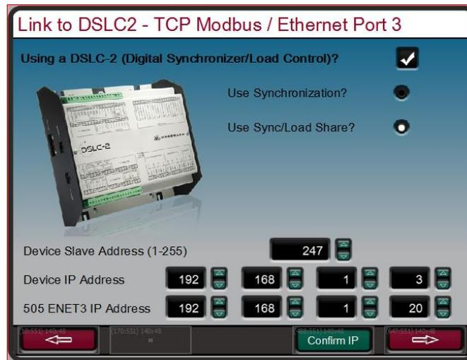
Figure 9-2. Configuration/Woodward Links/DSL2-2
