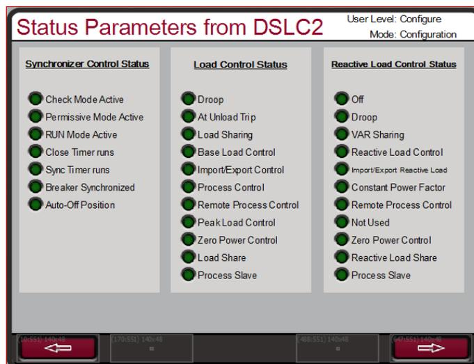
Figure 9-4. Service Screen - DSLC-2 Status Parameters
