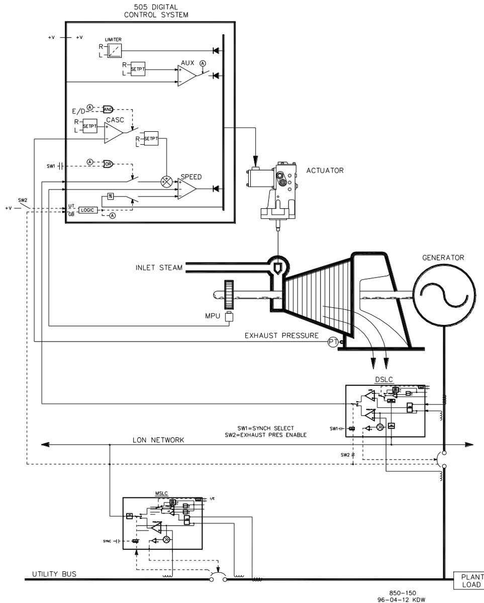
Figure 10-6. Import/Export Control or Exhaust Pressure Control with Isoch Load Sharing in Island Mode
