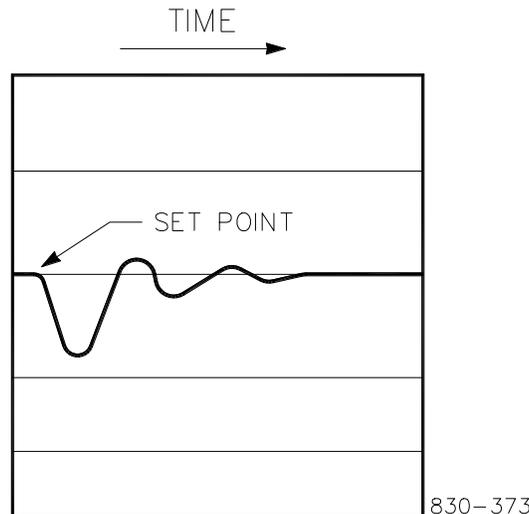
Figure 13-8. Typical Response to Load Change
