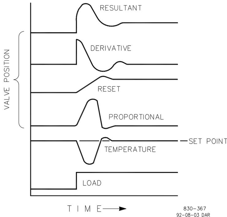
Figure 13-7. Closed Loop Proportional, Integral and Derivative Action
