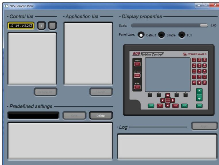
Figure I-8. Entering an IP Address to be Added to the Control List
