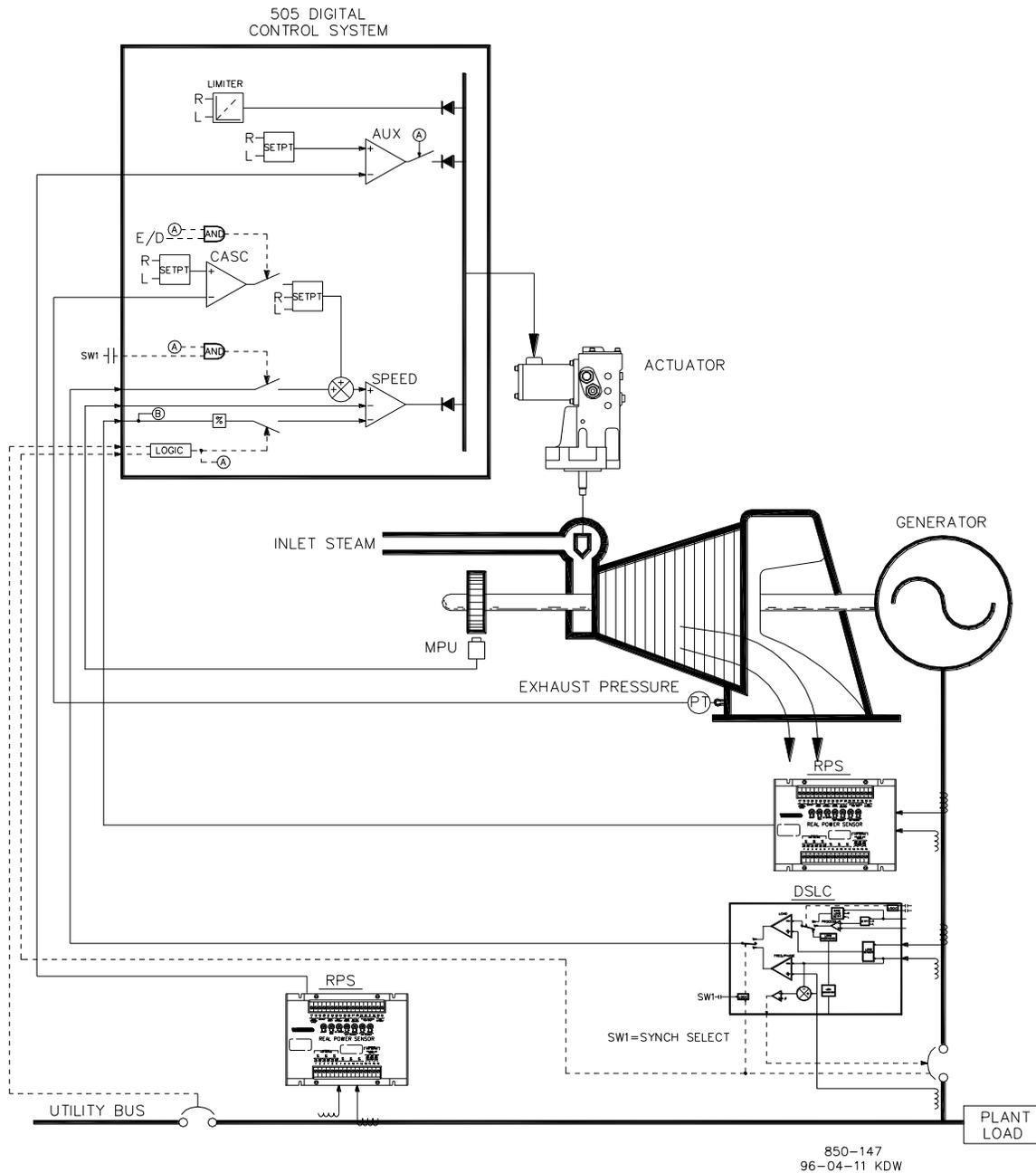
Figure 10-3. Exhaust Pressure Control with Generator Power Limiting and Plant Import/Export Limiting
