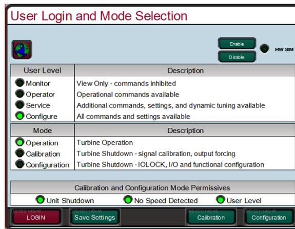
Figure J-1. HW Simulation Mode Access
