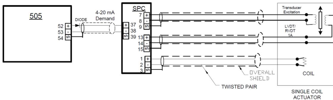
Figure 9-11. Interface to Servo Position Controller
