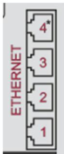
Figure A-4 Ethernet port 4 for DR communication link (redundant mode)
