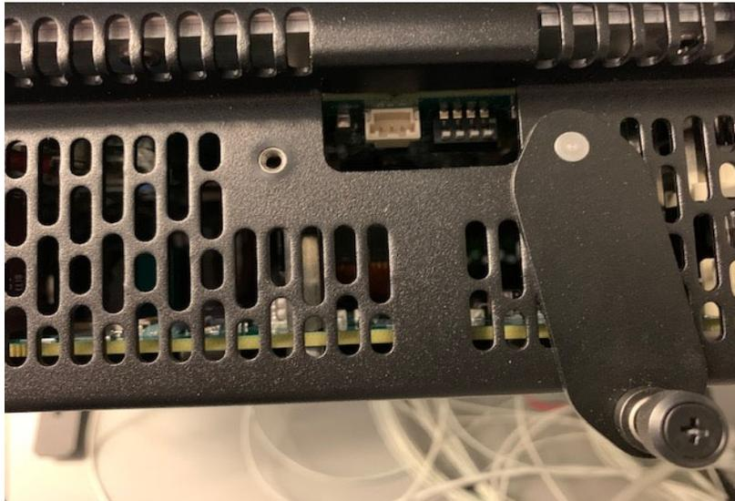
Figure A-1. Factory Default Settings of Switches (Simplex Mode)
