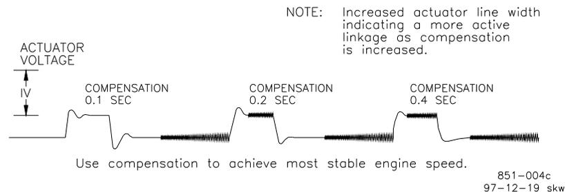
Figure 3-15. Typical Transient Response Curves
