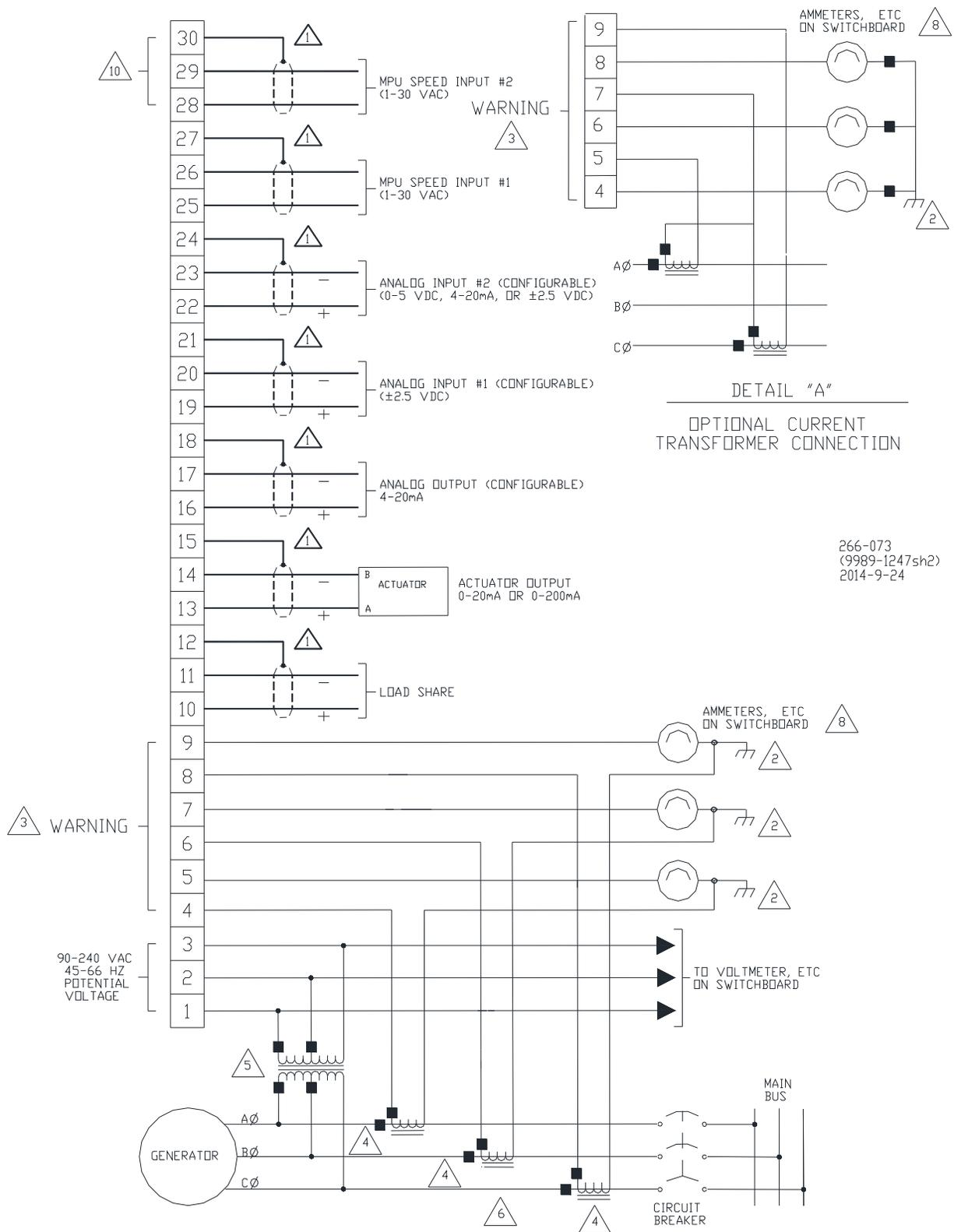
Figure 2-2a. 2301E-ST Plant Wiring Diagram (sheet 1)
