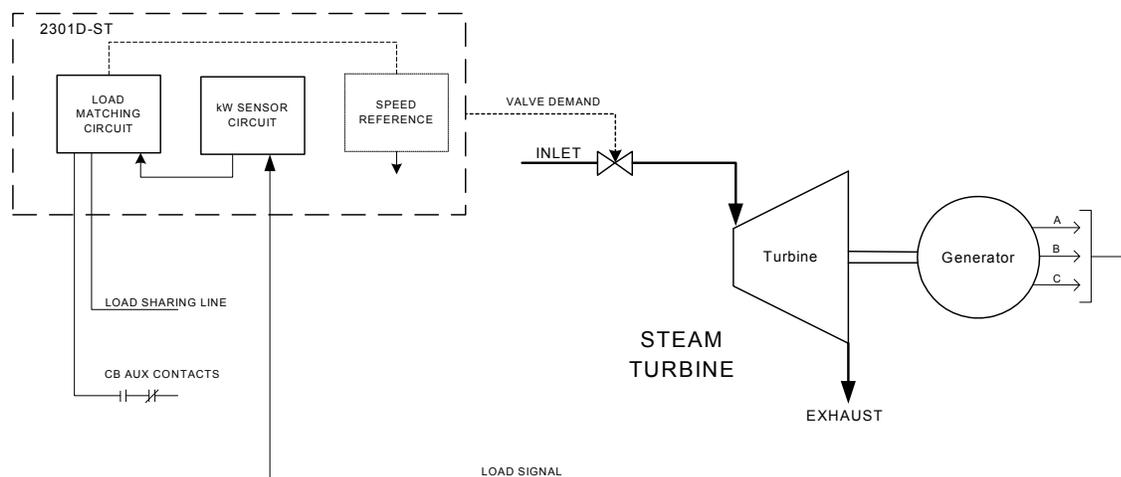
Figure 4-6. Paralleling System
