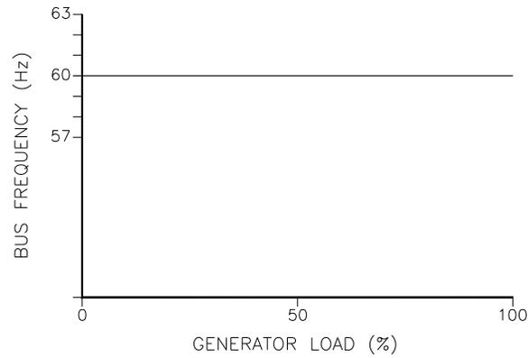
Figure 4-8. Isochronous Mode
