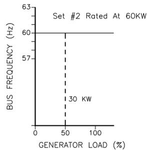
Isochronous Maintains Frequency and Load Swings
