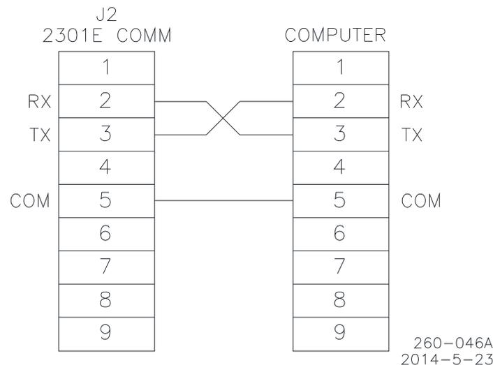
Figure 3-1. Null Modem Cable
