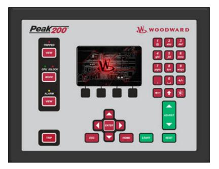
Figure 5-2. Peak200 Keypad with "Splash Screen"
