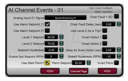
Figure I-12: Menu selection for Analog Input Start Permissive
