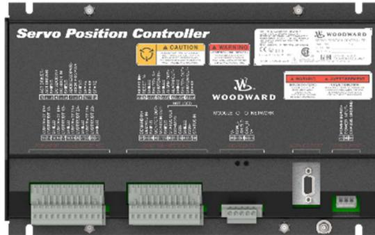
A Windows based service tool is used to configure the SPC, adjust tunables, and monitor parameters via a personal computer. For ease of service, SPC configurations can be done either while connected or disconnected to the unit. Once a configuration has been created, this program allows configurations to be uploaded and downloaded to other SPCs as desired.
