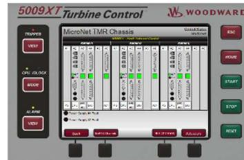
The control's PID-to-PID logic allows stable control during normal turbine operation and bumpless control mode transfers during plant upsets, minimizing process over or undershoot conditions. The 5009XT controller senses turbine speed via passive or active speed probes and controls the steam turbine through actuators connected to the turbine inlet steam valves.
