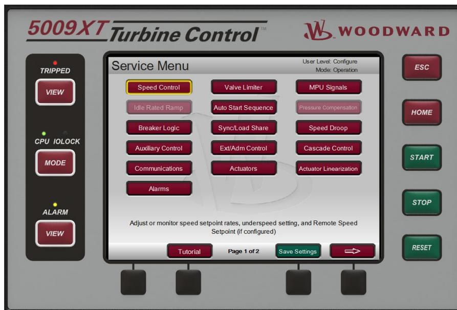
Figure 4-7. Service Menu showing “Speed Control” IN-Focus
