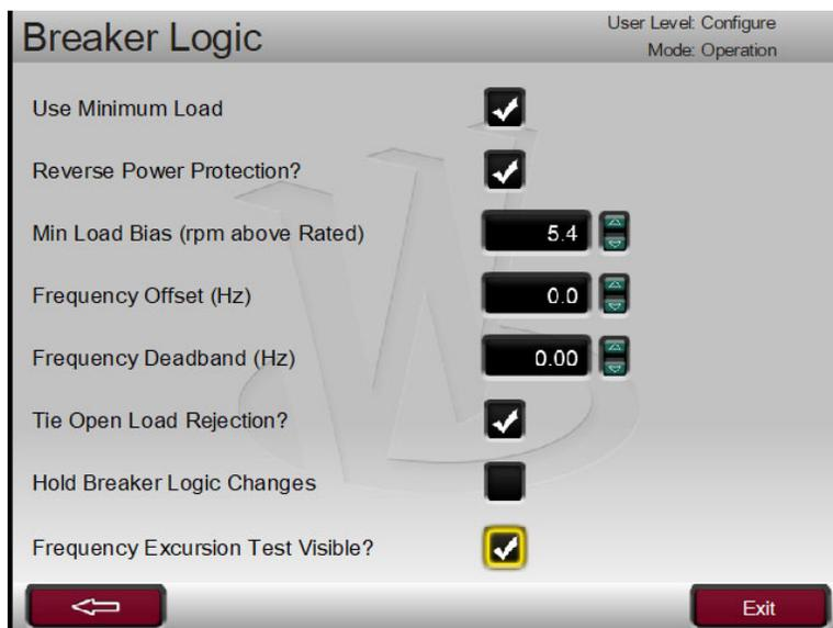
Once checked, press the Home key twice to return to the runtime home page. Then, in Speed Control, press the “More” softkey until the “Freq Test” is visible.
