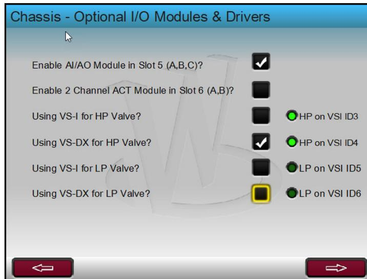
Figure 17-15. Example of VS-DX for HP and single VS1 for LP
