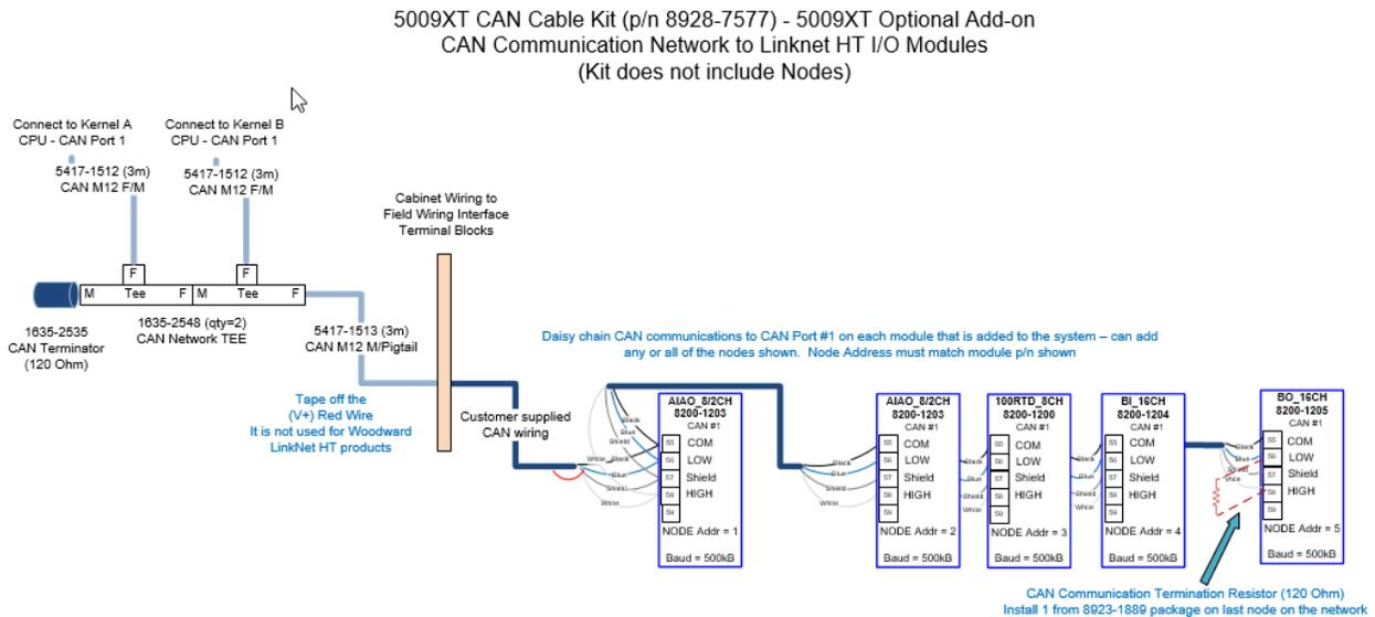
Figure 17-5. CAN wiring of Distributed I/O Network
