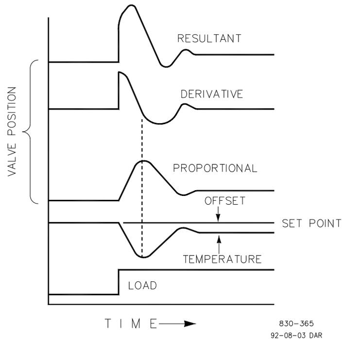
Figure 16-5. Closed Loop Proportional and Derivative Action
