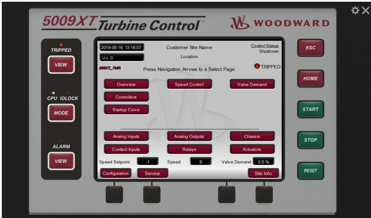
Figure L-13. Simple View of the 5009XT Tool
