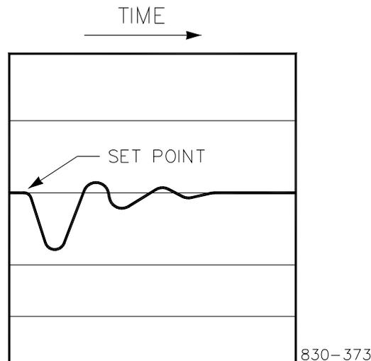
Figure 16-8. Typical Response to Load Change
