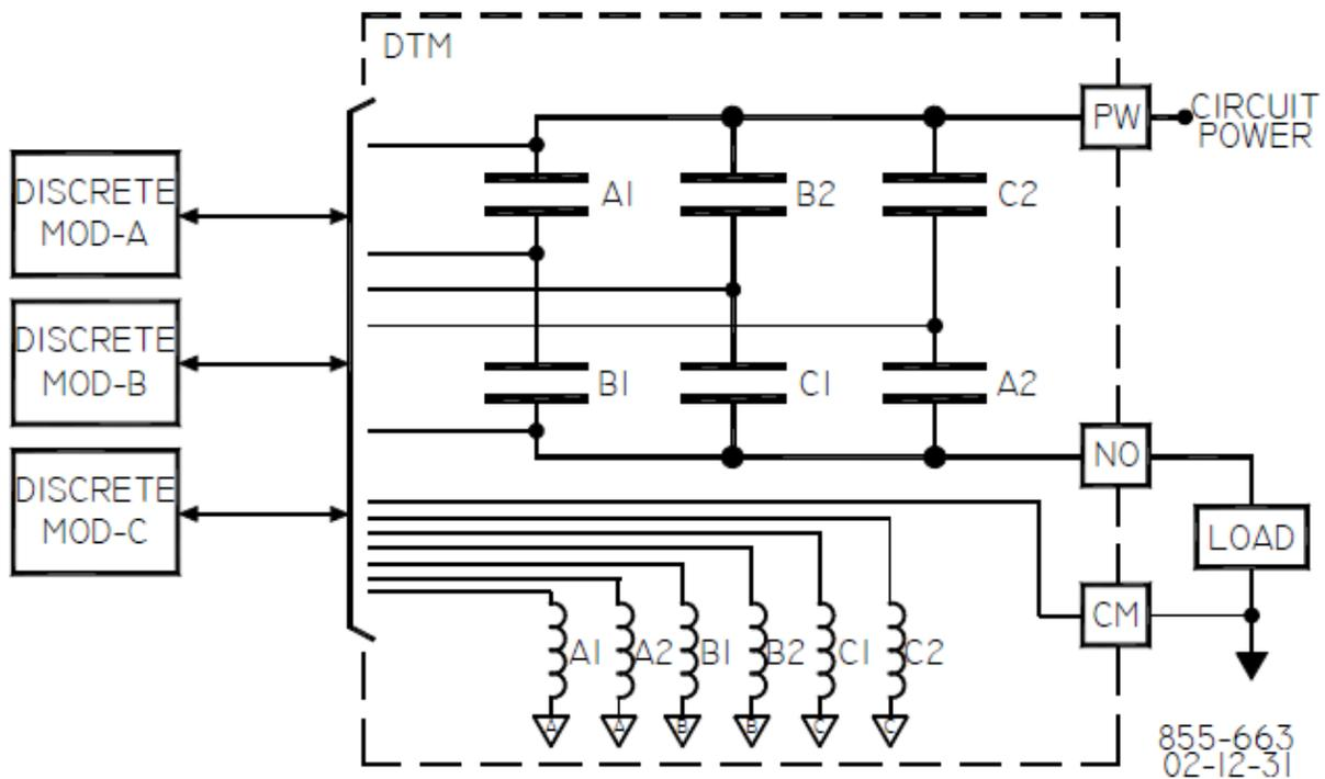
Figure 8-7. Fault Tolerant Discrete (Relay) Output
