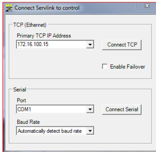
Figure I-5. SOS - Enter 5009XT TCP/IP address
