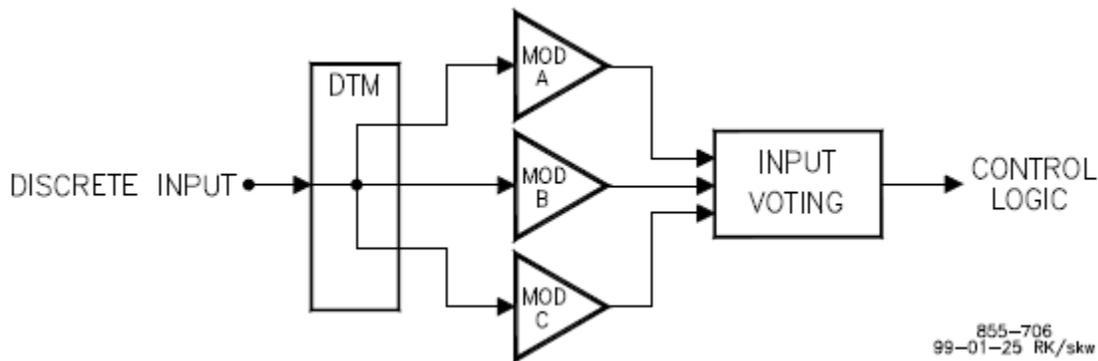
Figure 8-5. Fault Tolerant Discrete Input
