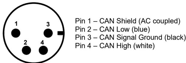
Figure 11-16. CAN Communication Ports (M8 male)
