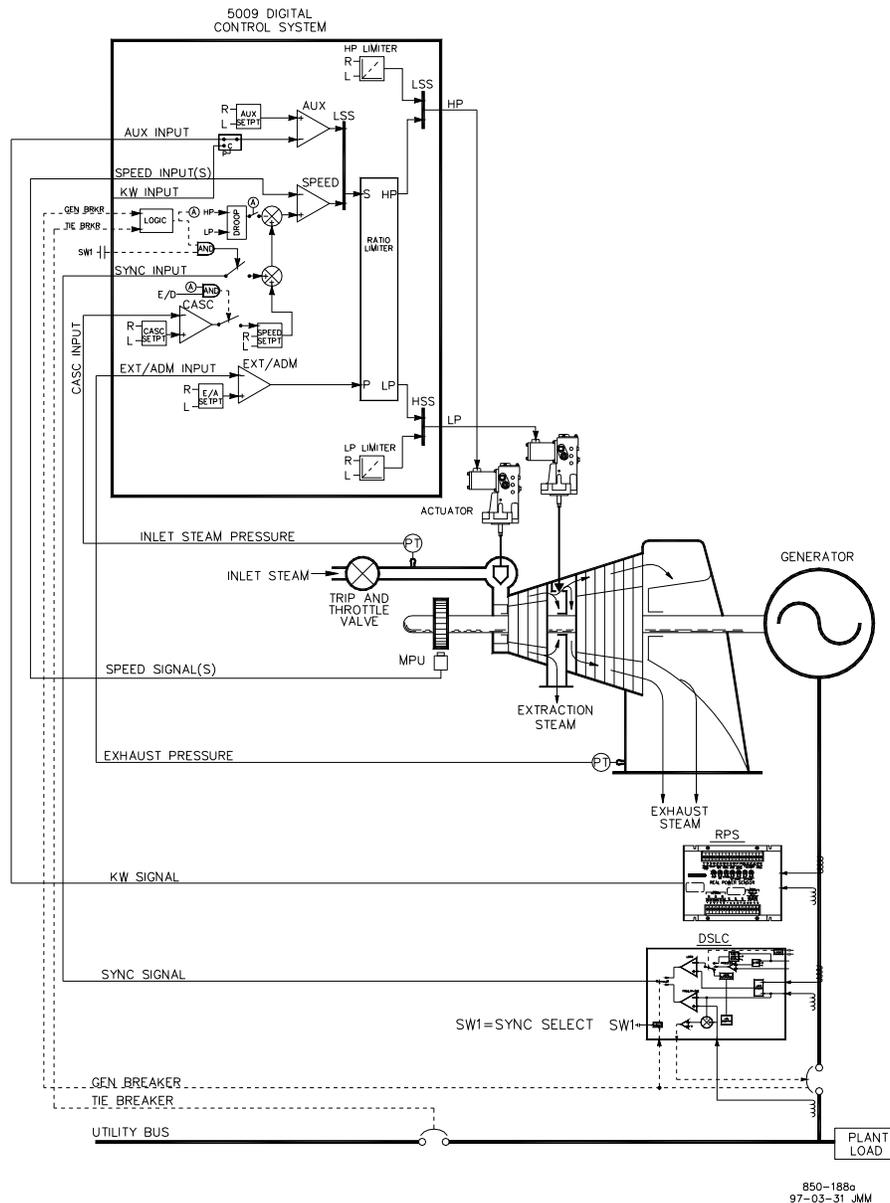
Figure 15-8. Inlet Pressure Control, Exhaust Pressure Control with Generator Power Limiting
