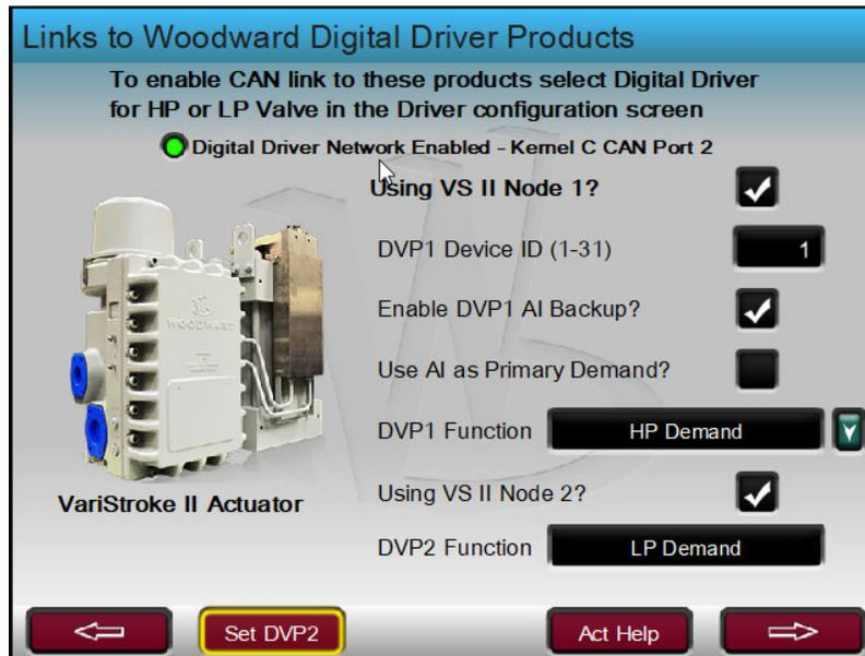
Figure 17-12. Configuration Screen for VS-II (1 or 2 Nodes)
