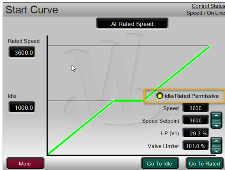
Figure 17-22. Start Curve Screen with Idle/Rated Permissive Used
