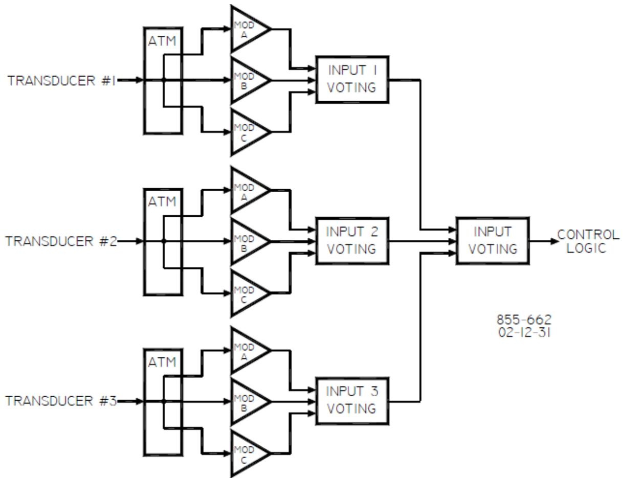
Figure 8-3. Fault Tolerant Analog Input
