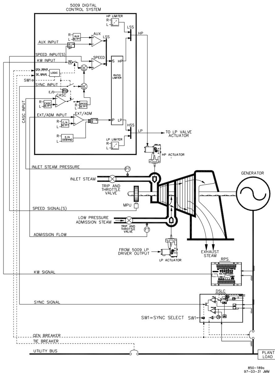
Figure 15-9. Admission Steam Turbine Control with Bootstrap Start-up
