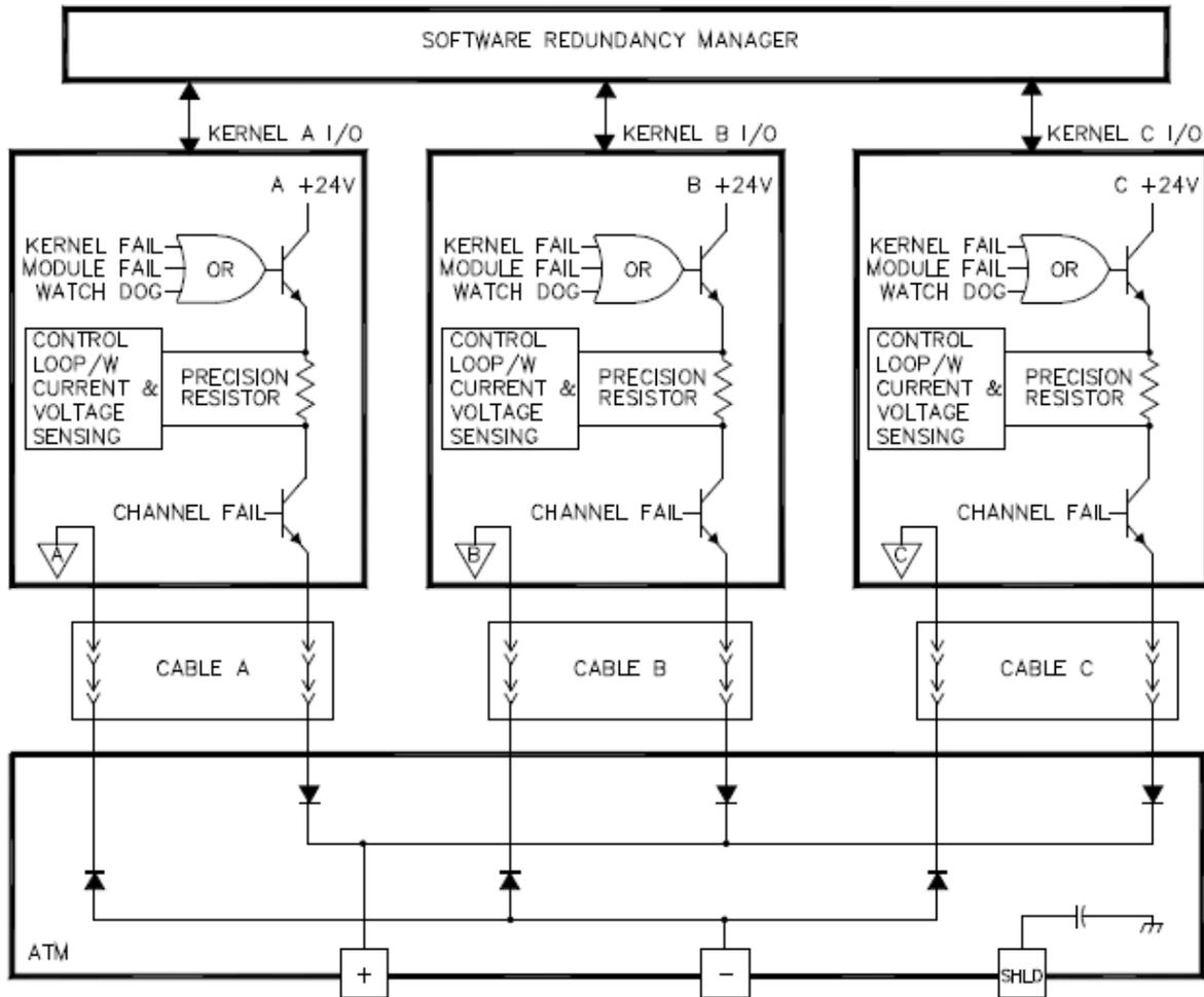
Figure 8-6. Fault Tolerant Analog Output
