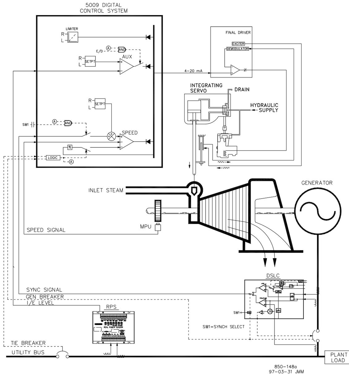
Figure 15-4. Plant Import/Export Control with DRFD Servo Interface
