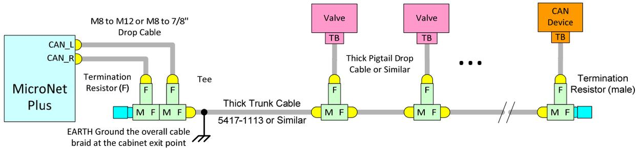
Figure 11-17. MicroNet to Valve CAN Interface
