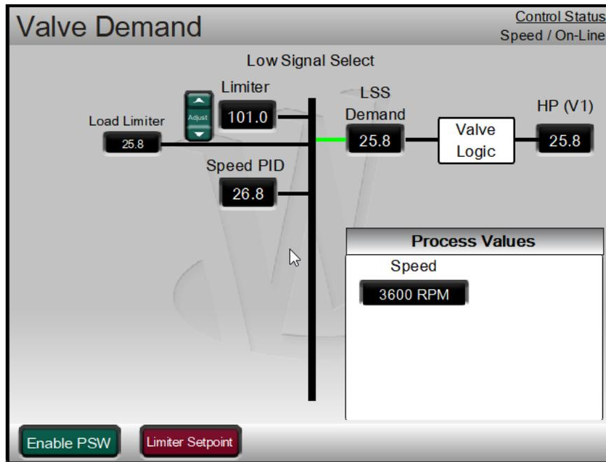
Figure 17-26. Valve Demand with Load Limiter is Active
