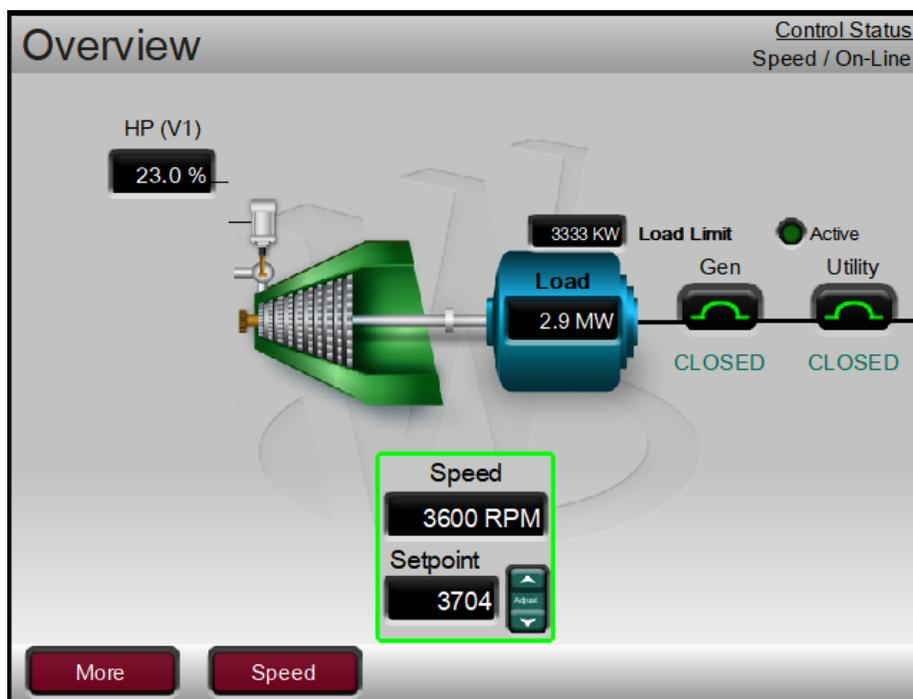
Figure 17-24. Overview of Load Limiter Enabled (Not Active)
