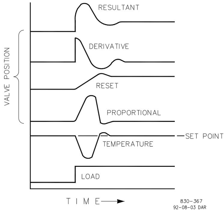
Figure 16-7. Closed Loop Proportional, Integral and Derivative Action
