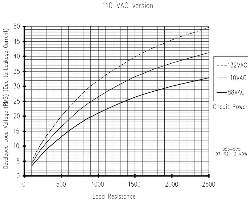
Figure 11-10. Latent Fault Detection Verification Graph—88–132 Vac Circuitry
