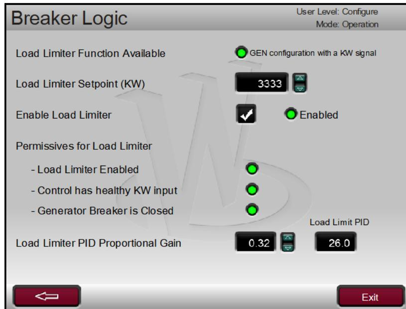
Figure 17-23. Service/Breaker Logic – Load Limiter Function Settings
