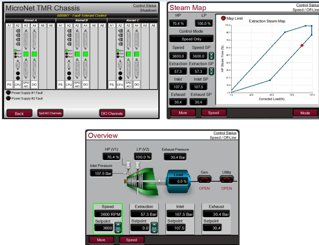
**5009XT Digital Fault Tolerant Control for
