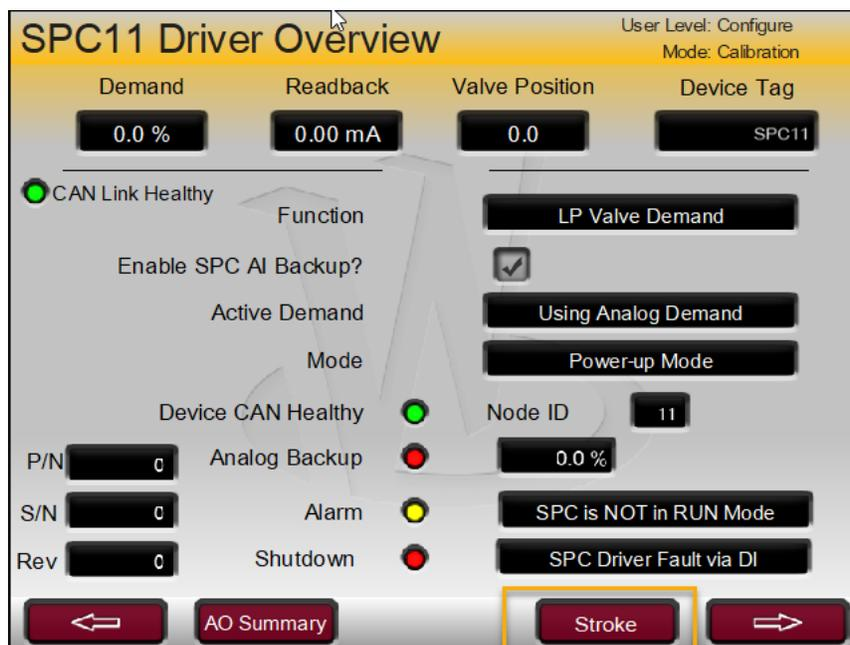
Figure 17-20. Access to Stroking of SPC Demand (Calibration Mode)
