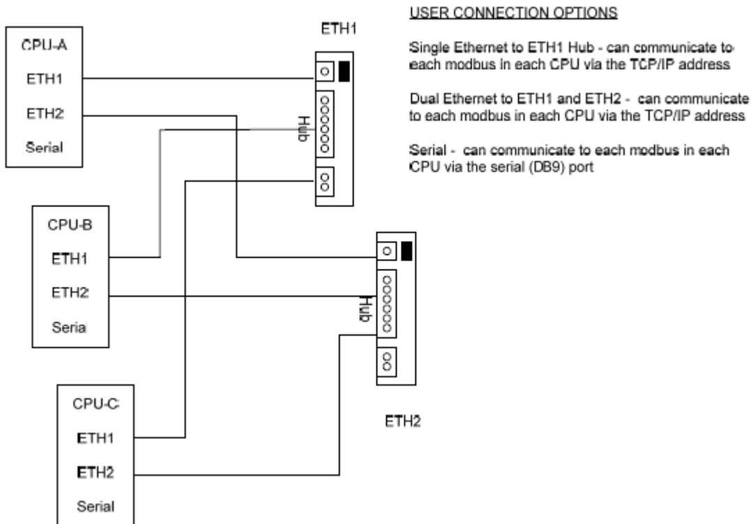
Figure 8-8. Fault Tolerant Modbus Communication Ports
