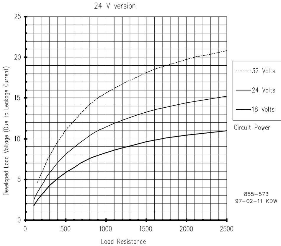
Figure 11-9. Latent Fault Detection Verification Graph—18–32 Vdc Circuitry
