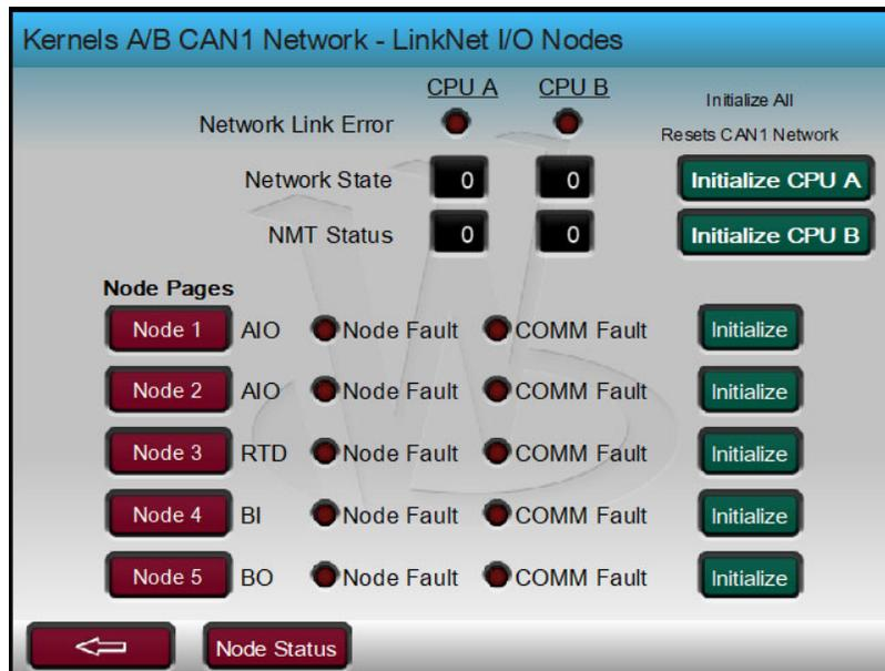
Figure 17-8. Distributed I/O CAN Network and Node Status
