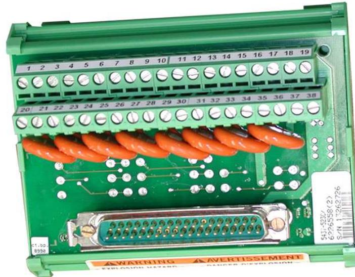
Figure 12-19. Analog Input FTM
