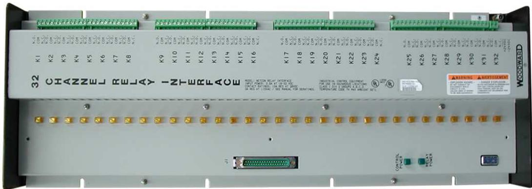
Figure 12-62. 32 Channel Relay Module
