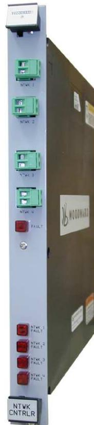
Figure 10-1. Four Channel LINKnet Controller Module
