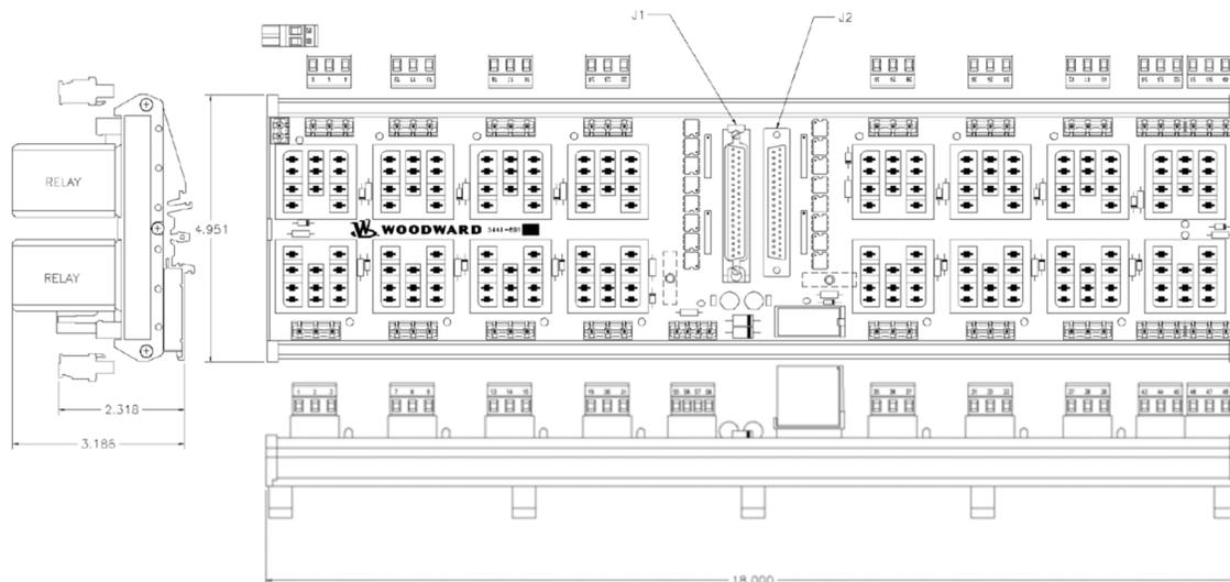
Figure 12-55. 16 Channel Relay Module (Phoenix Contact) Outline Dimensions
