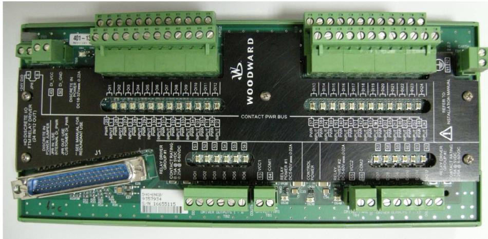
Figure 12-49. 24/12 Discrete I/O (with LEDs) FTM
