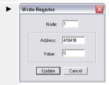
Fig. 333: Write register - enable the resetting procedure
